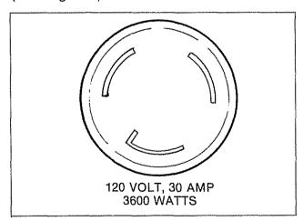
The outlet has a 30 amp or 3600 watt capacity. Do not attempt to run equipment requiring more than 30 amps or 3600 watts from the outlet.
